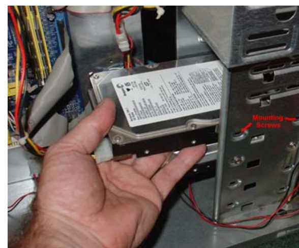
Figure 4. Installing the drive—carefully install your hard drive in a spare bay.
