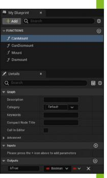
Figure 4: Interface classes don't let us add any code in the Interface itself - it is up to the class attached to deal with that. We can only deal with entry/exit points within the Interface class.
